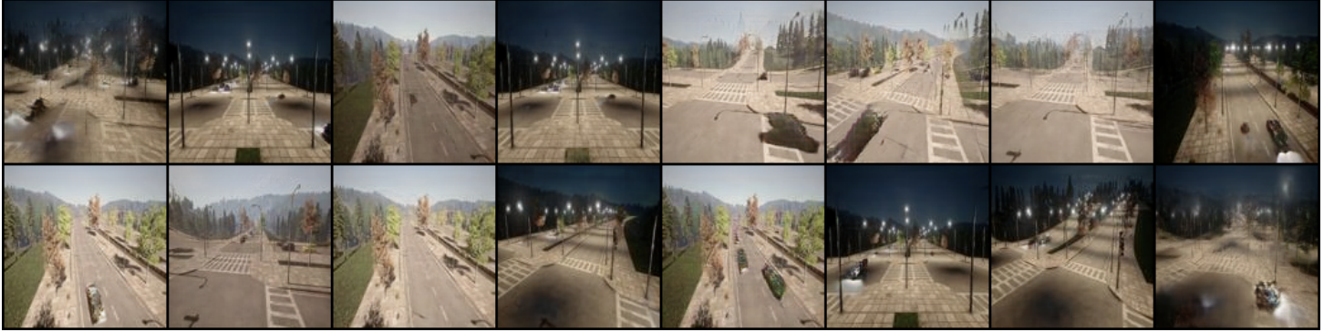
Figure 5.5: Samples generated by a WGAN-GP model trained with Digital Twin images of size (128,128). Parameters : [Batchsize = 64, iter = 90.000, dataset_size = 25.000images]
