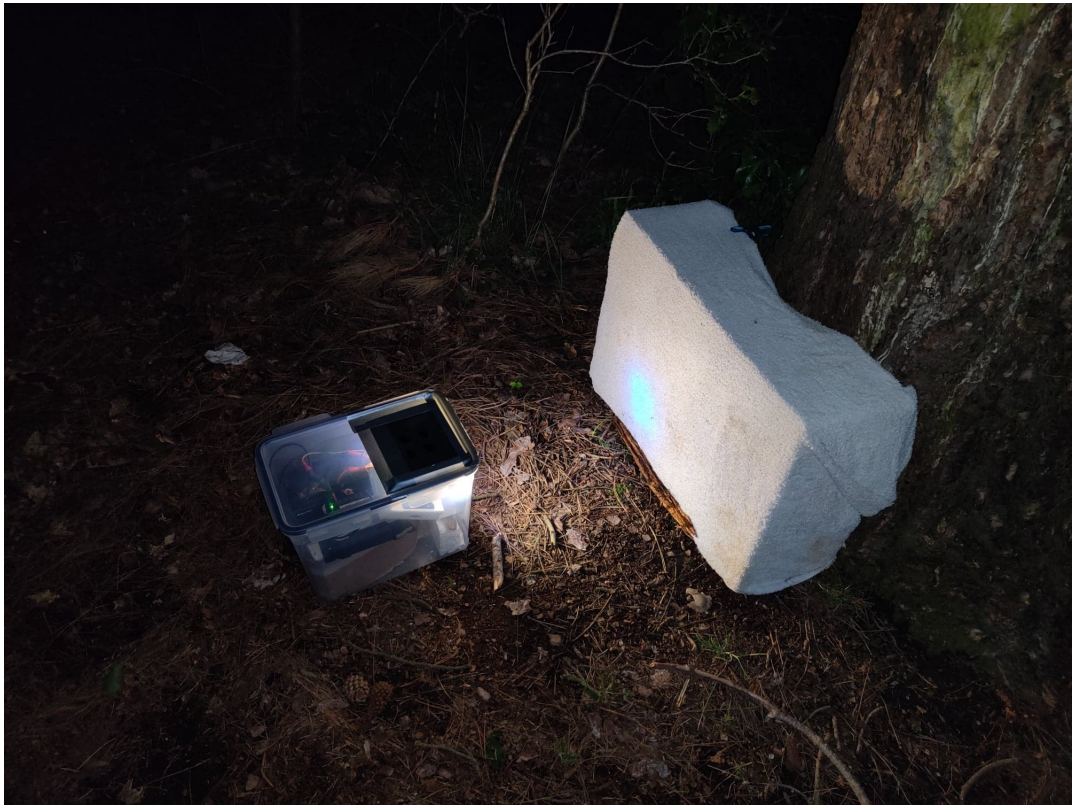
Figure 4.6: A picture of our trap in action, attracting insects on a white drape.
