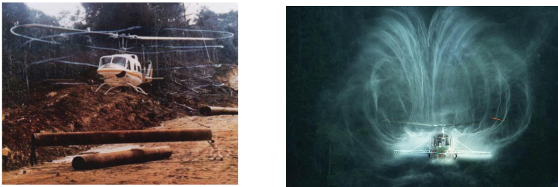
Figure 1: (left) Blade tip vortices of a helicopter in hover [1] and (right) Vortex State Ring visualisation [2].
