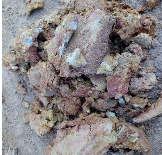
Figure 4.26: Hydromorphic traces observable in a deep sandy horizon overlaying the clay layer.
