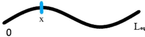
Figure 2.11: Representation of a linear chain within the Doi and Edwards model. The first extremity of the chain is located at the point 0, and the other extremity is at a distance L_{eq} from the point 0. A segment of the tube situated at a distance x from the extremity 0 is indicated in blue.
