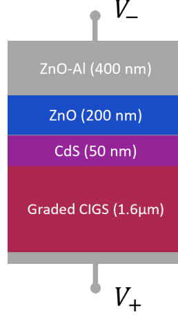
Figure B.2.1: SCAPS model of the reference CIGS cell. The back contact represented in grey has its metal work function aligned with the Fermi level of the adjacent CIGS (Flat-band parameter in SCAPS).
