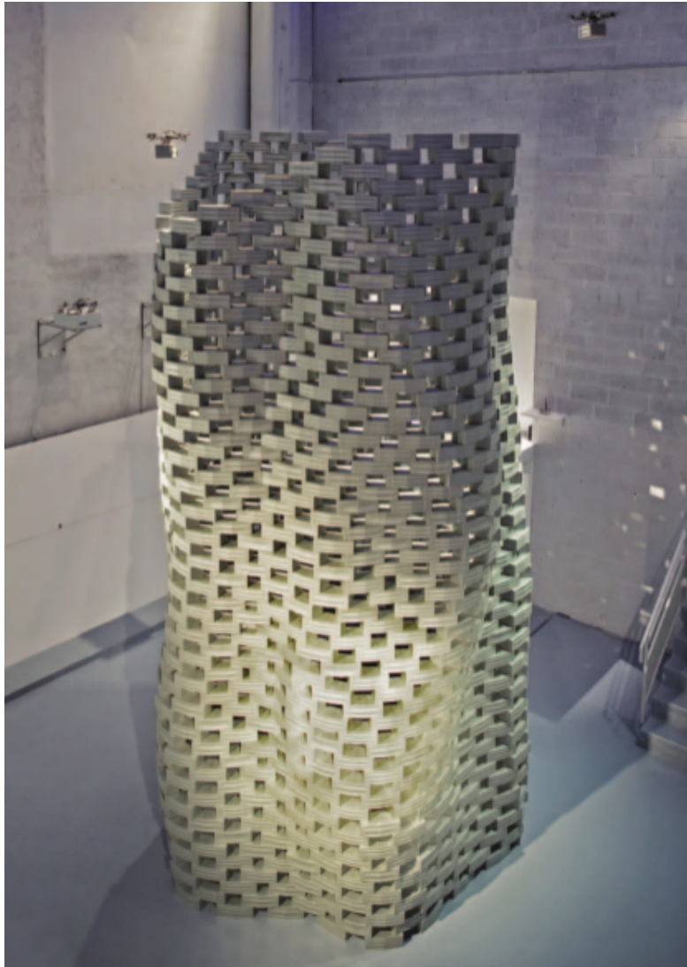
Figure 1.8: 6m-tall tower composed of 1500 foam blocks, built by four autonomous quadcopters during a real-scale experiment in France in 2011 [11].
