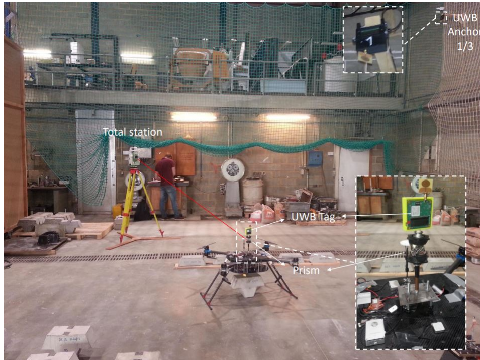
Figure 1.7: Overview of the complete project (except the camera) with : the total station on the left (pointing at the prism), a zoom on one of the three UWB anchors at the top right corner, a zoom on the prism + the tag mounted on the drone at the bottom left corner and finally the "middle-sized" testing drone at the bottom center of the picture.
