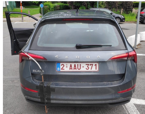
Figure A.4: Copper pipe attached to the framework of the car. All the
