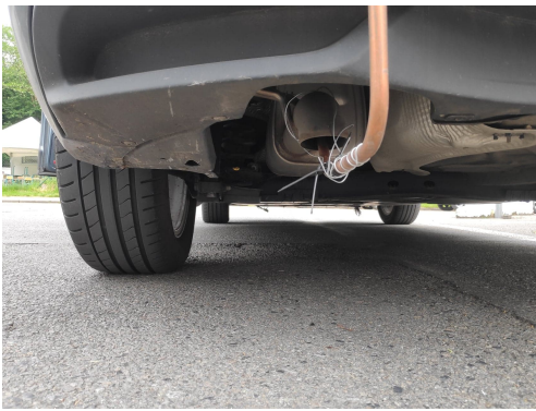
Figure A.3: Copper pipe attached to the exhaust.
