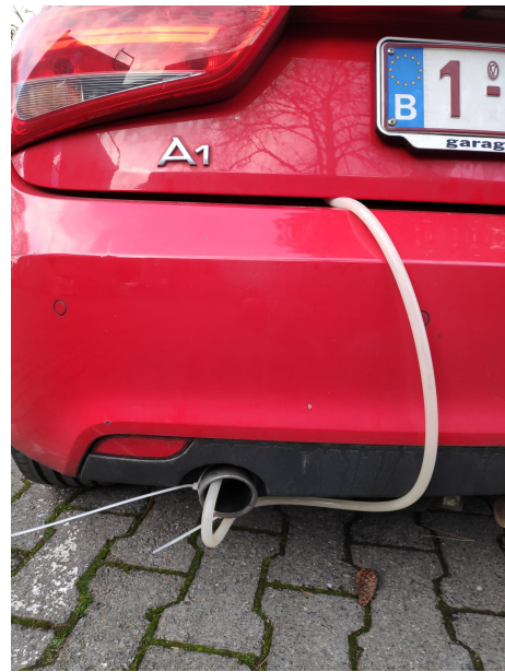
Figure A.2: Hose directly put in the exhaust.
