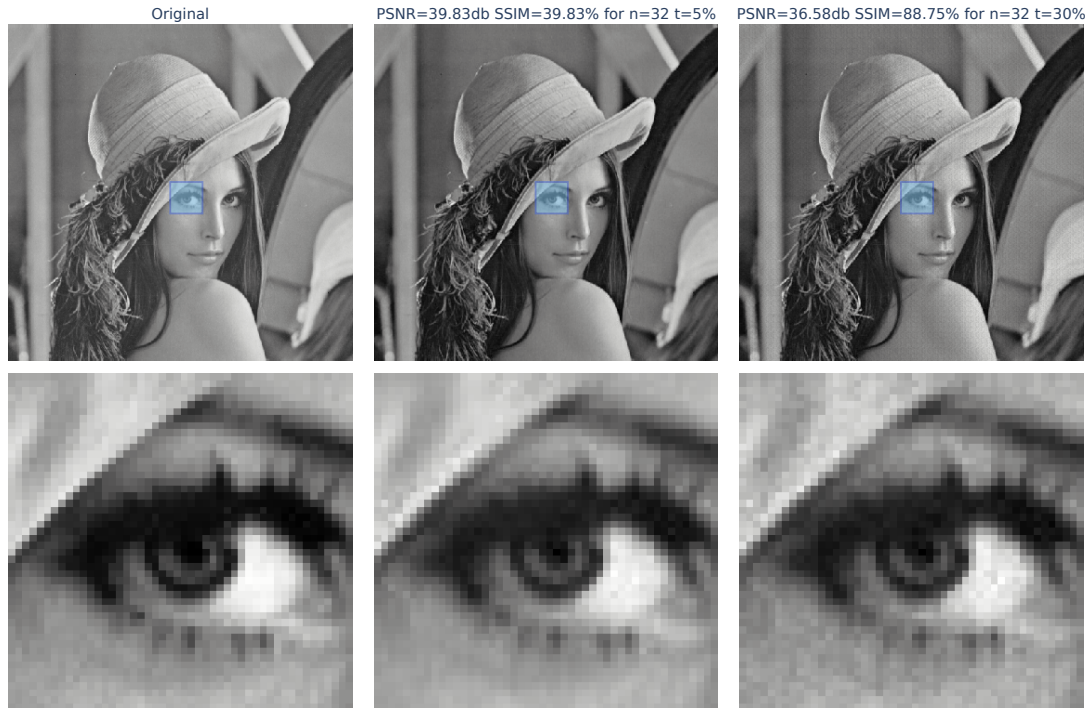
Figure 3.13: Original image and 2 compressed decompressed images with 2 bits approximation and n = 32 . The middle image has t = 5\% , the third has t = 30\% . The second row is a zoom on the blue box of the full size images.
