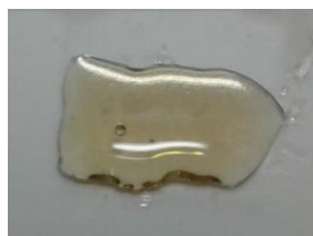
Figure 22: Aspect of the cured network of thioplast G131 + PEGDE 500 g/mol
