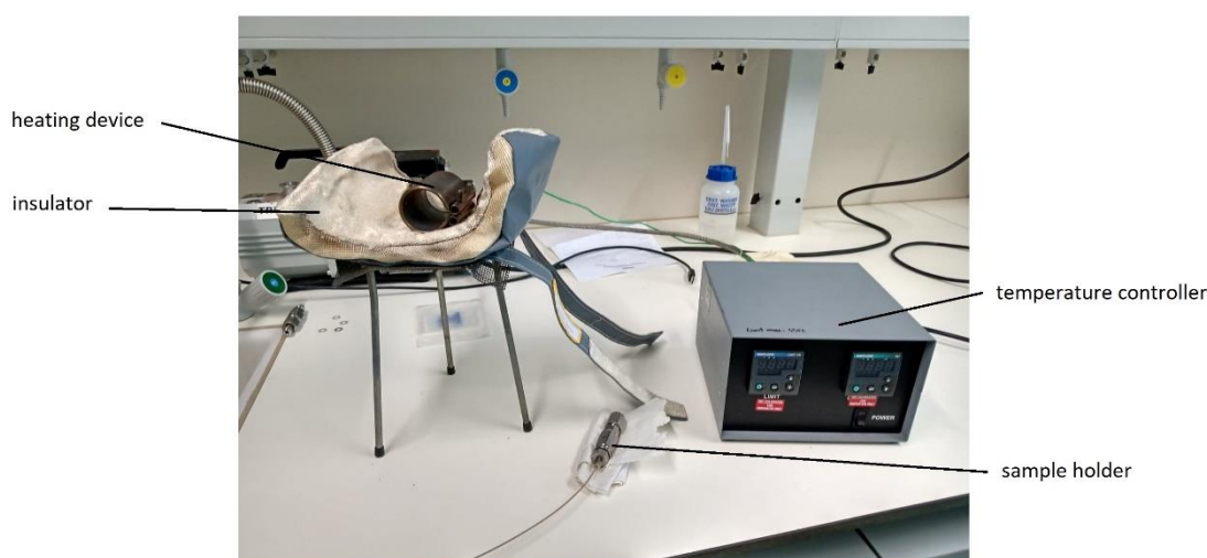
Figure 7 : Electronic heating device used for in situ activation in WGT method.
