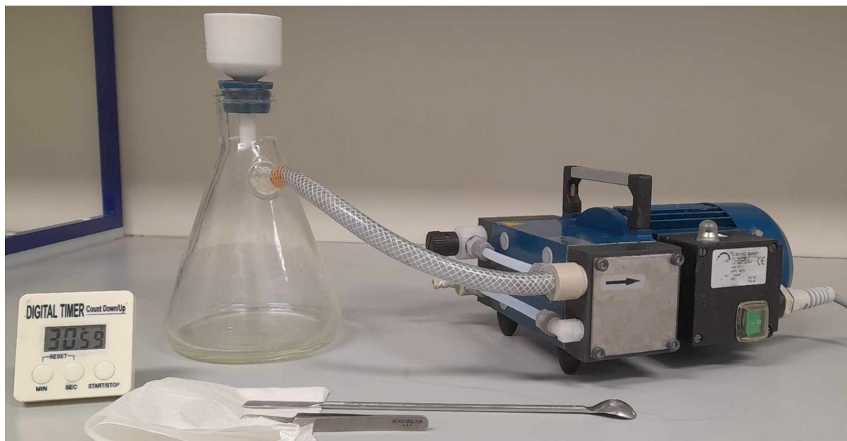
Figure 17: Setup for membrane impregnation.
