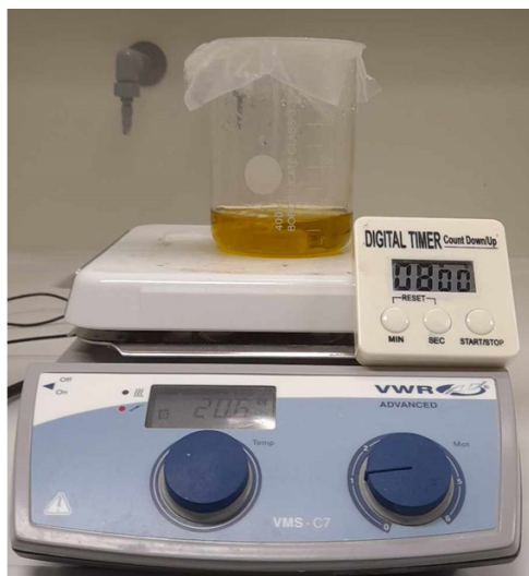
Figure 16: Setup for membrane coating.
