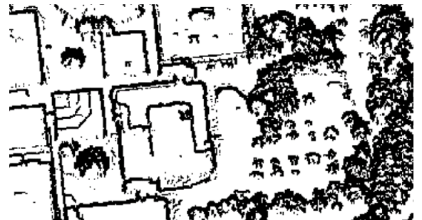
Figure 3.8: Shadow raster for a tolerance of 80% and a zoom on the roof of the De Serres building
