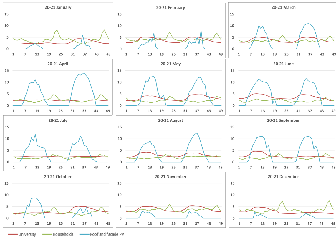
Figure 4.7: Load curves of the roof and facade production compared to the consumption of UCLouvain and Louvain's households in [MWh]
