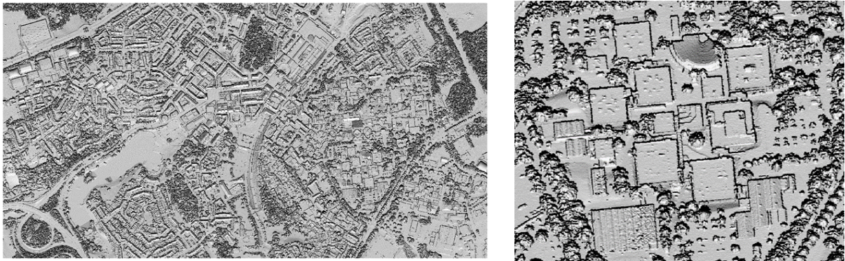
Figure 3.5: Hillshade raster for DSM and solar position of the 20 th of April at 12:00 and zoom in on the buildings in Place de la Croix du Sud
