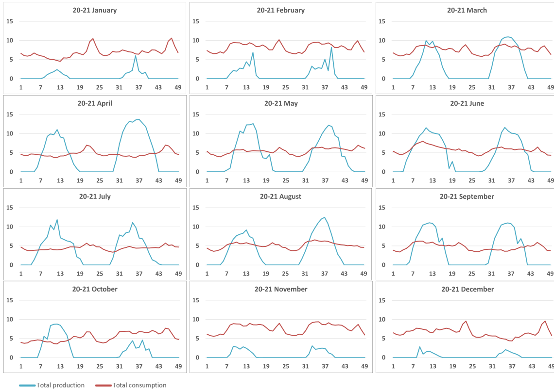
Figure 4.8: Load curves of the total of the roof and the facade production compared to the total consumption of UCLouvain and Louvain's households in [MWh]
