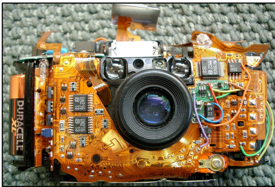
Figure 2: Olympus stylus type camera without the cover (manufactured by Olympus). The flexible PCB can be seen wrapped around the object. This allows for a single PCB to be used instead of a combination of a mother and children set of boards. Image by Steve Jurvetson on Flickr. [10]
