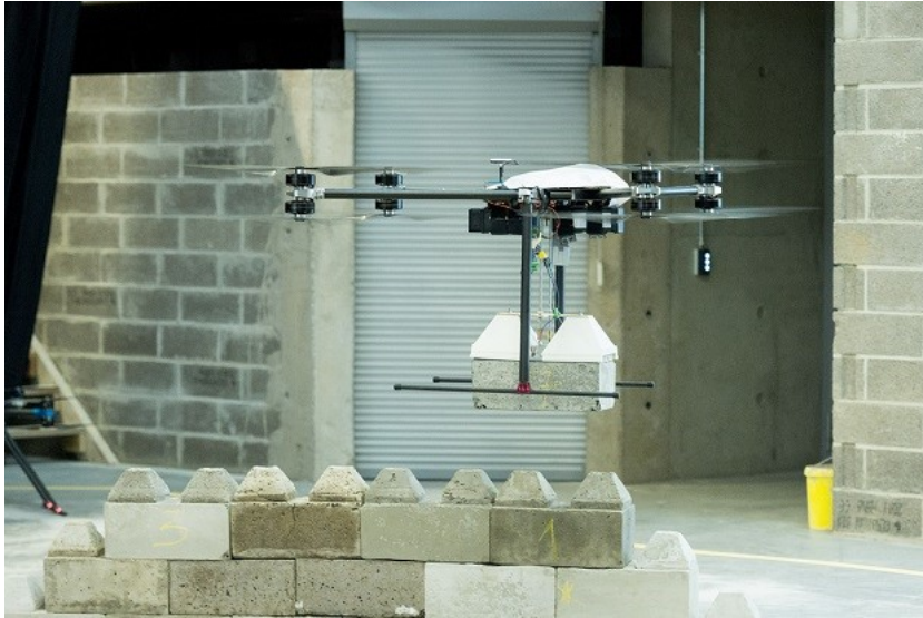
FIGURE 3.4 – Mur de Dricks 2
