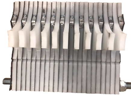
Figure 6.2: All fixed knives assembled together with 3D-printed blade spacers
