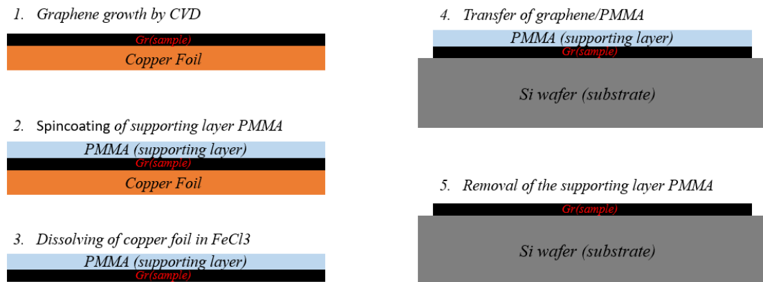
Figure 20: Graphene Transfer steps
