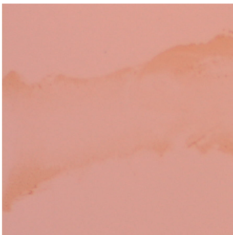
Figure 21: Oxidation of copper because of the presence of water between substrate and graphene
