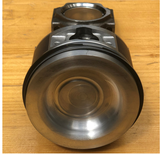
Figure 2.3: Piston head after machining.
