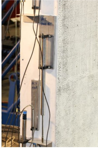
Figure 6.6: Exemple of the setup of LVDTs on a concrete wall from a previous test at the LEMSC [22]
