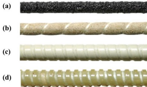
Figure 2.2: FRP rebars with different types of surface finishes: a) sand coating b) sand coating with exterior wound fibers ribs c) ribs and d) ribs [9]
