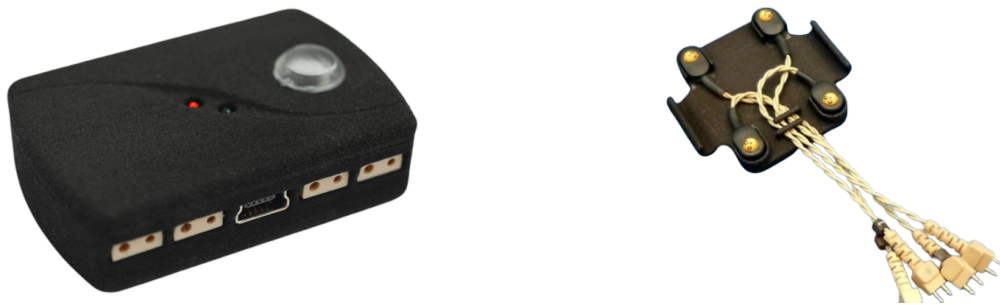
Figure 3.3: Drive box and LED markers [3]
