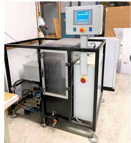
Figure 7: Pulsating jet erosion test (PJET) used at Sonaca for water droplet erosion tests. Figure (a) shows a schematic representation of the working principle from Keegan et al. [9] while Figure (b) is a picture of the actual machine.
