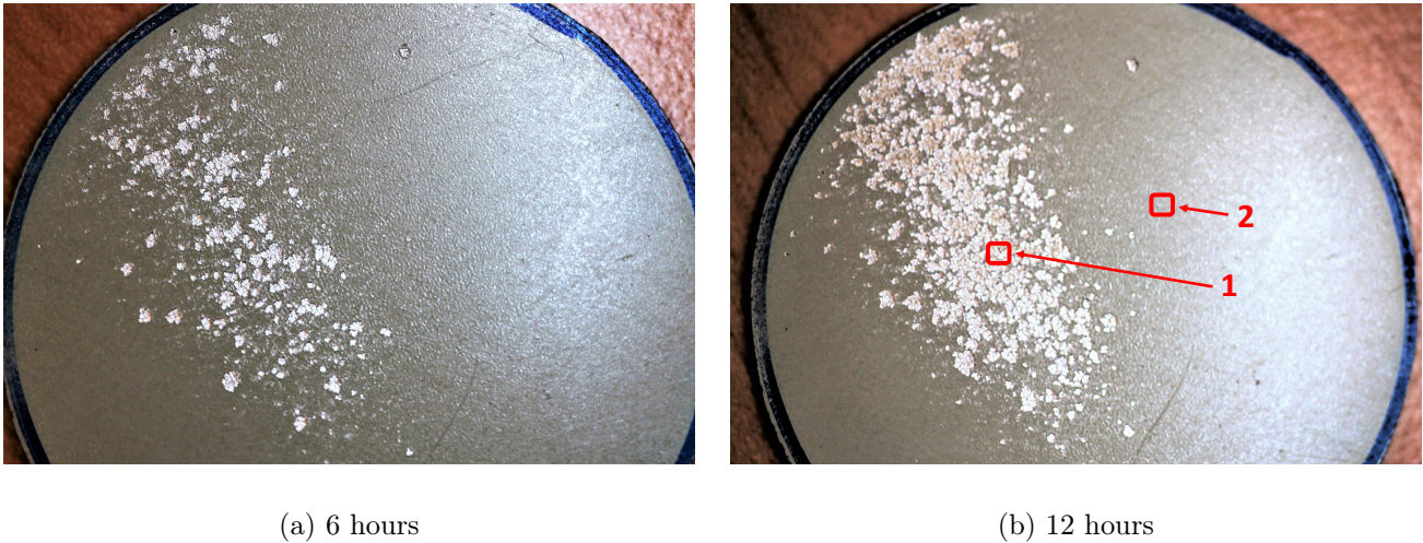
Figure 18: Macro images of the chromium anodized Al2024 with an epoxy coating sample, exposed for (a) 6 hours and (b) 12 hours to erosion at standard conditions in the WAREER.
