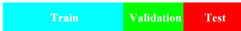
Figure 3.3: The training set is used to fit the models, whereas the validation set is used to estimate prediction error for model selection, and finally the test set is used for evaluating the generalization error of the best performing model [4].
