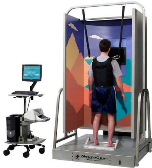
Fig.1. The Equitest® system (Neurocom International, Clackamas, Oregon) composed of a dual-force platform, a visual panorama and a computer. ( https://www.interempresas.net )
