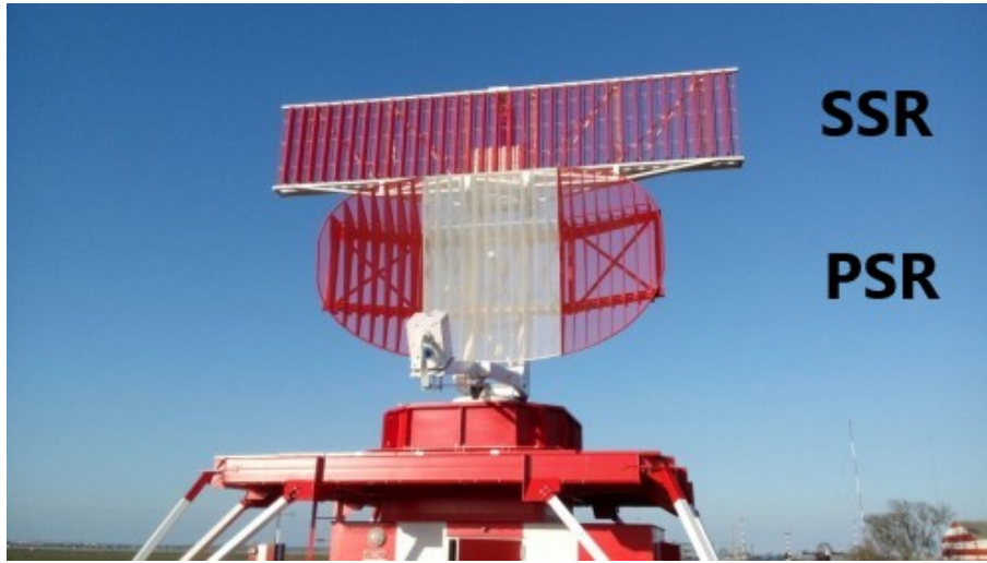
Figure 2.1: Secondary Surveillance Radar on top of a Primary Surveillance Radar [Azimut, 2021]
