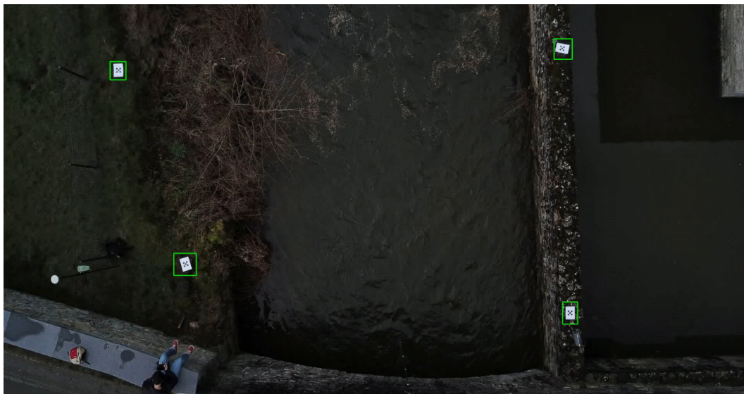
Figure 7.16: First frame of a video that needs stabilization. The stabilization is performed using the four green rectangles.
