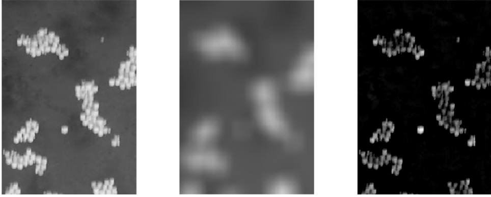
Figure 7.6: Intensity High-Pass filter. Figure from [49]
