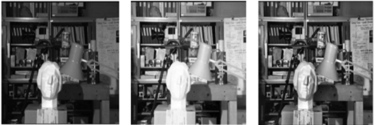
Figure 7.9: From left to right, original image, after AHE filter and after CLAHE filter. Figure from [96]
