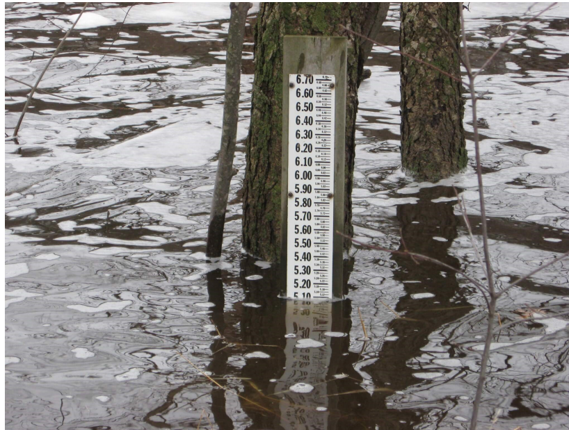
Figure 2.4: Example of staff level gauges. Figure from [14]
