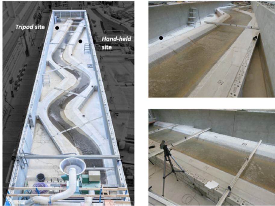
Figure 4.3: Flume use in the experiment of Carrel to evaluate Discharge application. Figure from [74]
