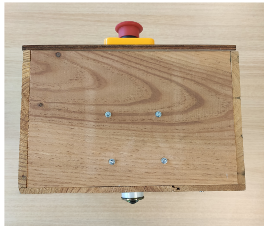
Figure C.2: Front of the robot: the emergency-stop button is placed above the freebear wheel
