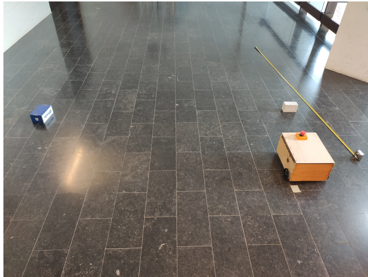
Figure D.9: Turning motion experiment: two boxes were placed, one for each time the robot would be parallel to the tiles. The distance was measured between these two boxes to obtain the diameter of the achieved circle
