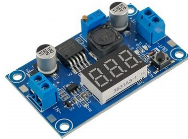
Figure 3.12: Buck converter used
