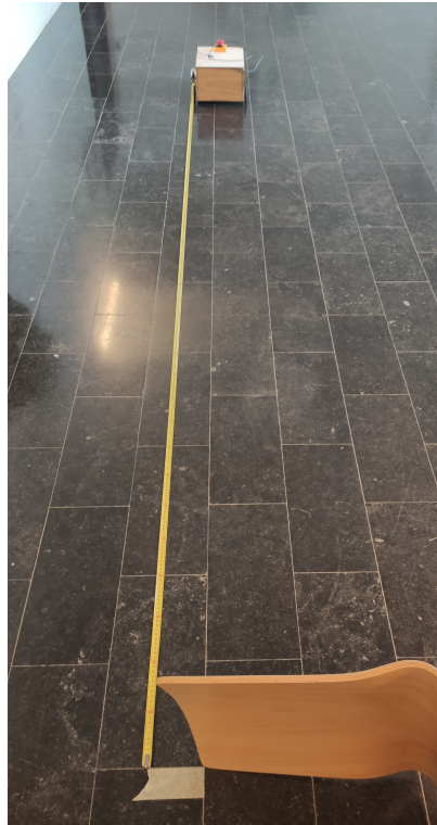
Figure D.2: End of the first experiment: the distance is measured between the front of the robot and where its front originally was
