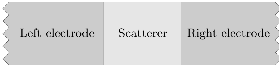
Figure 2.2: Schematic of a device for quantum transport. The device region (here called "scatterer") is sandwiched between two electrodes. The left and right electrodes are considered semi-infinite. Adapted from [24] .
