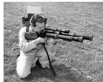
Figure 3.1: Hughes Aircraft Company engineer, Rod Smith, aiming the Colidar mark II, the world's first commercial LiDAR [70]
