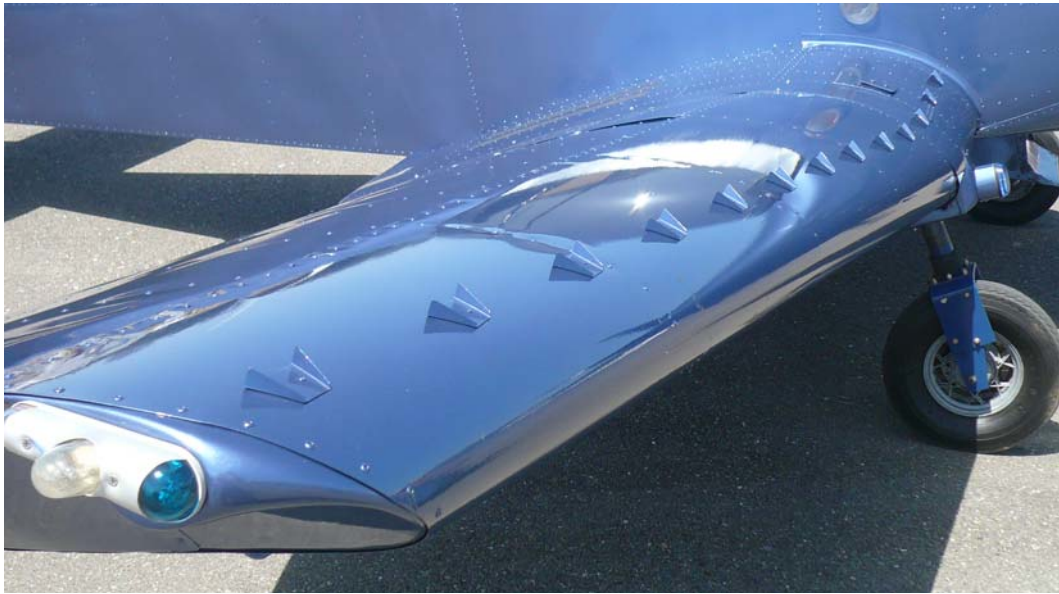
Figure 6: Example of passive air flow control actuator : Vortex generators on a Zodiac CH 601 HD wing
