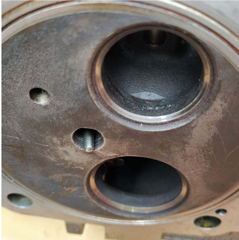
Figure 2.11: Possible configuration of the GP mounting in the cylinder head.
