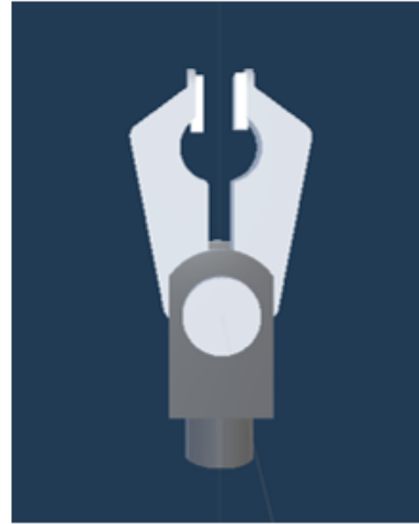
Figure 3.17: Modelling of the Greifer prosthesis designed with FreeCAD software.
