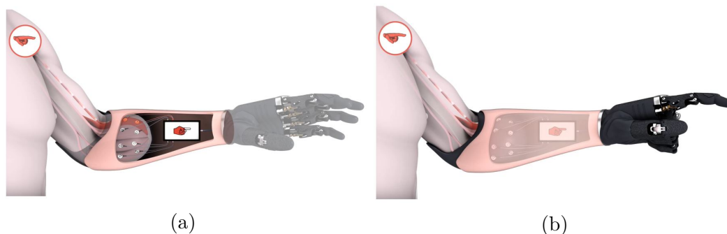
Figure 2.10: Processing of the information captured by the electrodes (a), followed by the execution of the movement by the prosthesis (b) [41].
