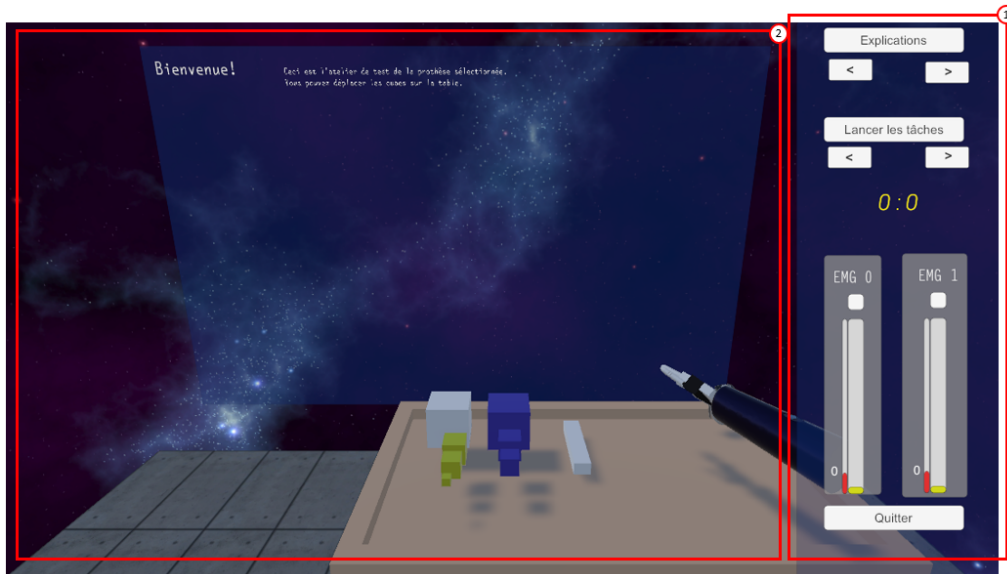
Figure 3.14: Test Room : point of view of the operator. The subject point of view is visible in the background (2), while the dashboard (1) is only visible for the operator.
