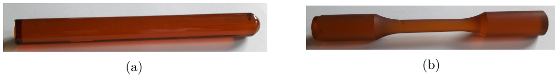
Figure 3.2: Pictures of a) cured resin from a thin glass test-tube mold and b) an unpolished dogbone sample.
