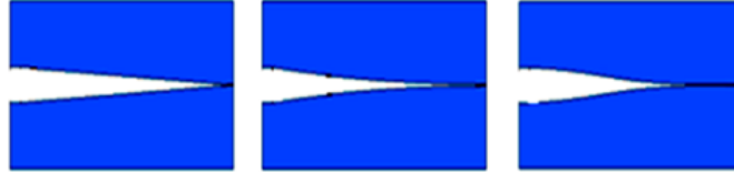
Figure 3.21: Representation of 3 different tapered lines structure (from left to right): exponential, triangular and Klopfenstein from [33]
