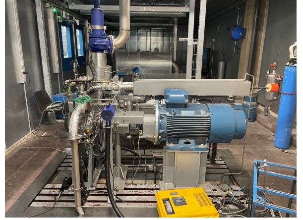
Figure 3.7: UCL HCCI research engine
