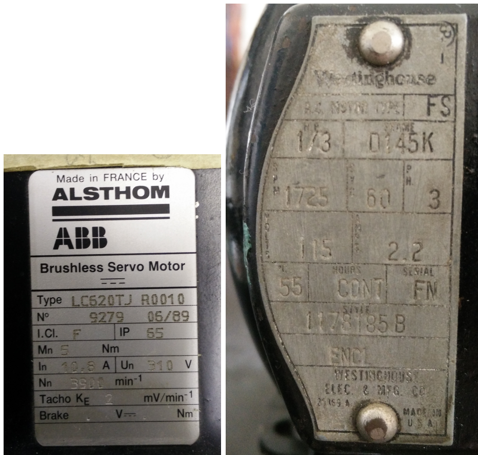
Figure A.8: Name plate of the synchronous (left) and asynchronous (right) machine
