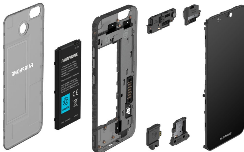
Figure 8: Exploded view of the Fairphone 3 and its components (Android Authority, 2019)
