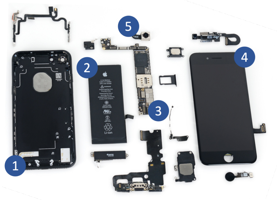
Figure 2: Exploded view of the iPhone 7 (iFixit, 2016)
