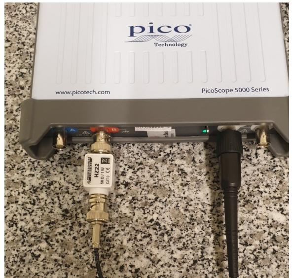
Figure 6.1: On the left: Current probe Tektronix CT1. On the right: PicoScope 5000 Series USB oscilloscope
