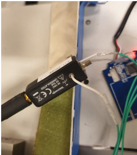
Figure 6.1: On the left: Current probe Tektronix CT1. On the right: PicoScope 5000 Series USB oscilloscope
