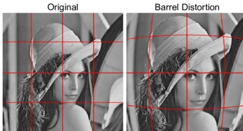
Figure 4.6: Barrel distortion photo taken by a fisheye lens for Lena 10
