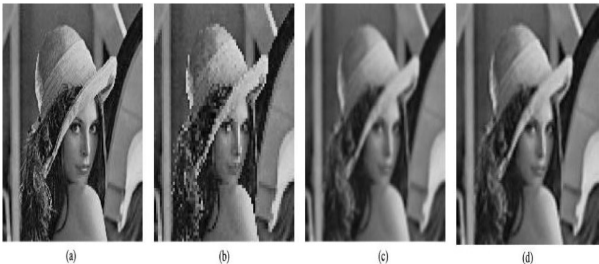
Figure 4.11: (a) original image of lena, (b) nearest neighbour method, (c) bilinear method, (d) bicubic method
