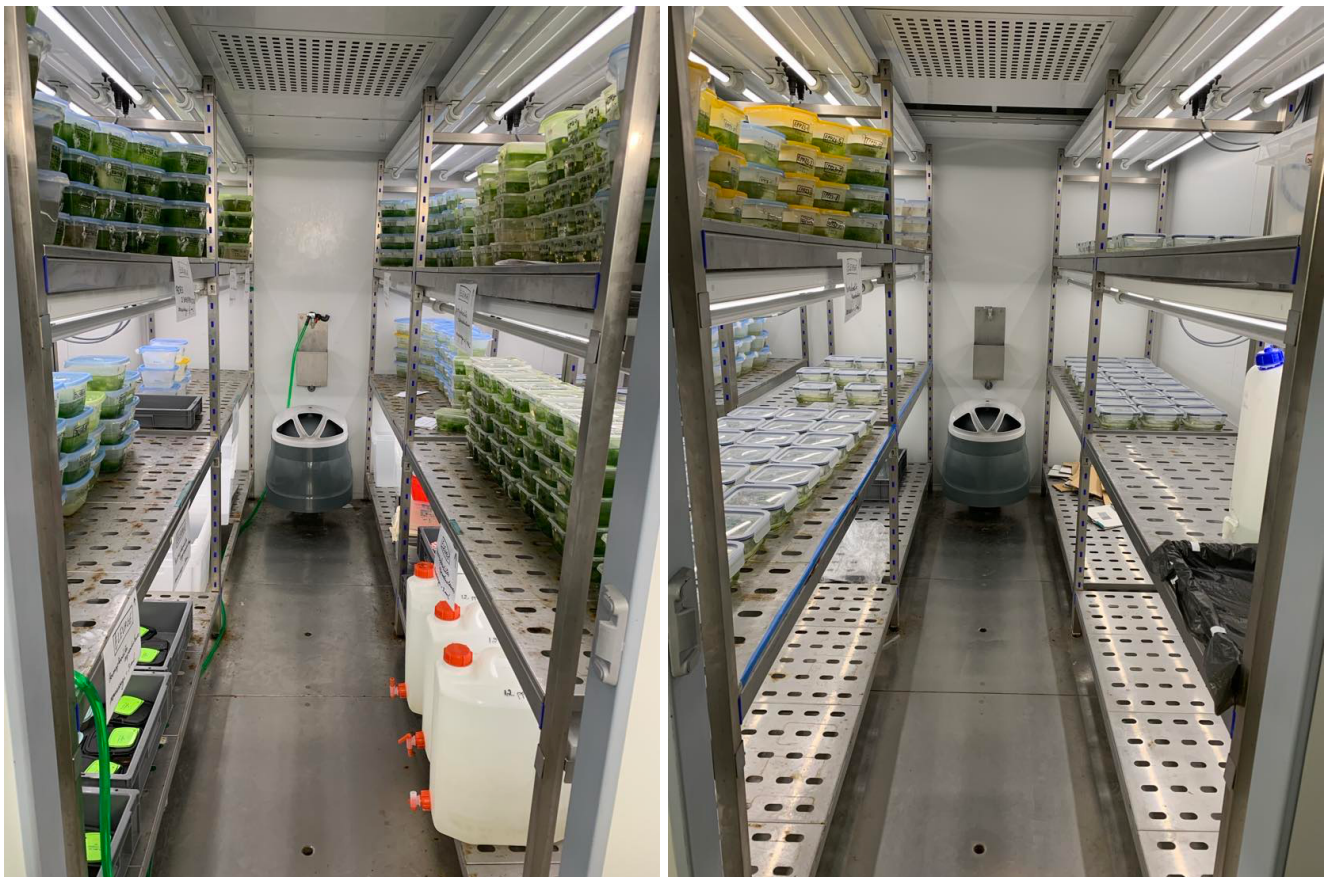
Figure S1: Incubators where the fish and the eggs were raised under laboratory conditions. Temperature is set to 25°C, and a photoperiod of 12:12 light:dark is applied. Fish are split following their original population and their age. © Gauthier Alexandrescu.
