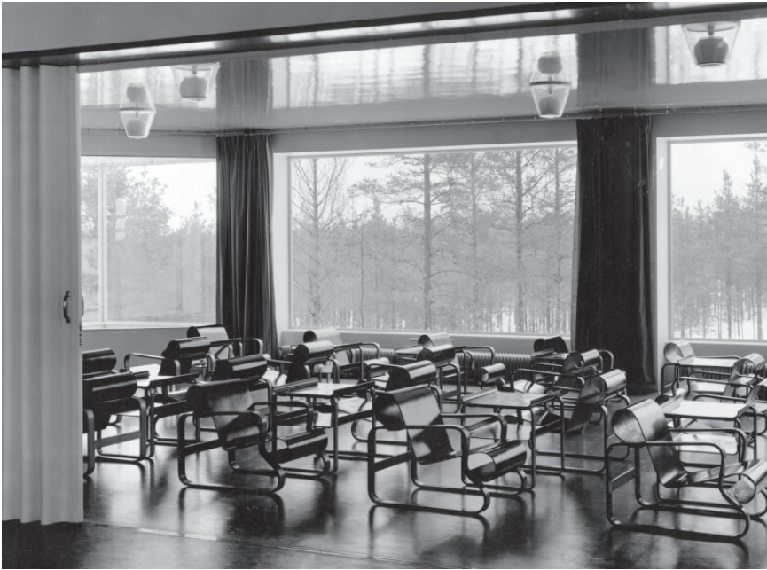
Fig. 3 - Architecture used as a tool to immerse the patient in positive distractions; reflective ceiling to reflect natural light, curtain partition allowing flexibility of space, large opening towards the forest, movable chairs. Tuberculosis Sanitarium by Alvar Aalto
