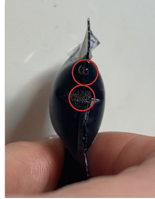
Figure 11.3: Leak detector bubbles on a pouch sealed at 230°C for 15s.
