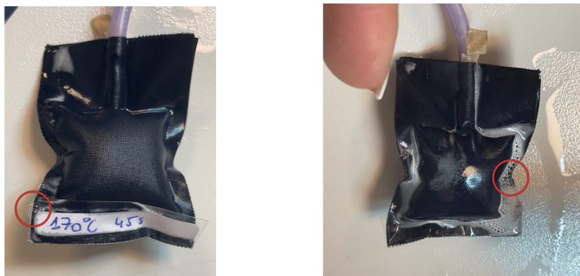
Figure 11.1: Leak detector bubbles on both sides of a pouch sealed at 170°C for 45s.
