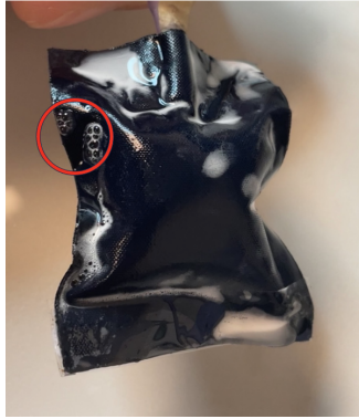
Figure 11.2: Leak detector bubbles on a pouch sealed at 200°C for 45s.
