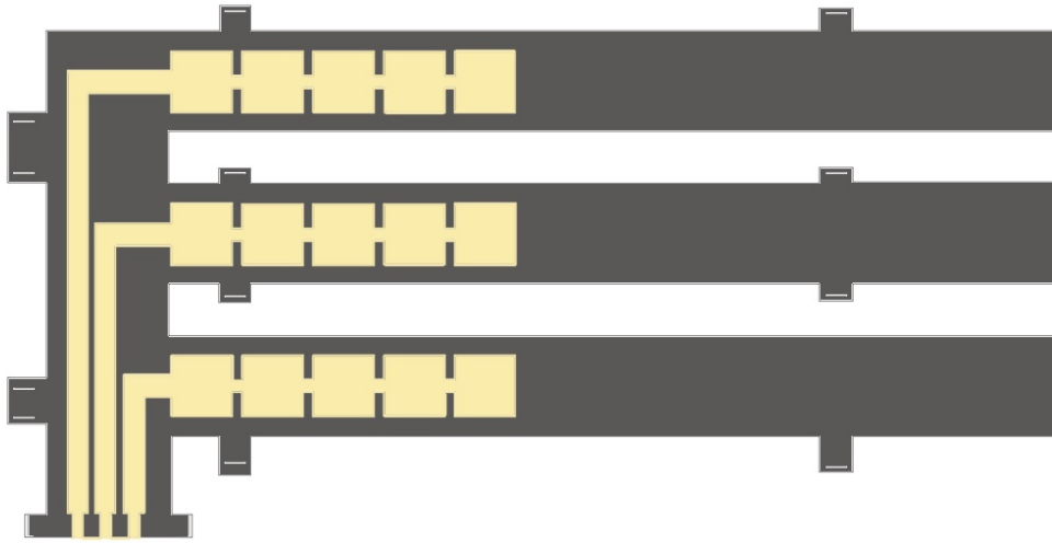
Figure 9.5: The design of the heat-sealable and intermediate layer used for the pneumatic bands conception by Schara et al.. Notches external to the bands main bodies are added in order to facilitate their alignment during the fusion process. Overflowing heat-sealable layer is intended for further fixation system on the leg.
