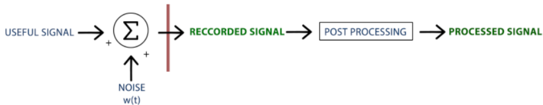
Figure 10: Listening trial (1): Illustration of source noise, added to the useful signal in an additional way. Noise can be too added in further step as during recording session induced by material, or noise induced by a not well suited preprocessing.
