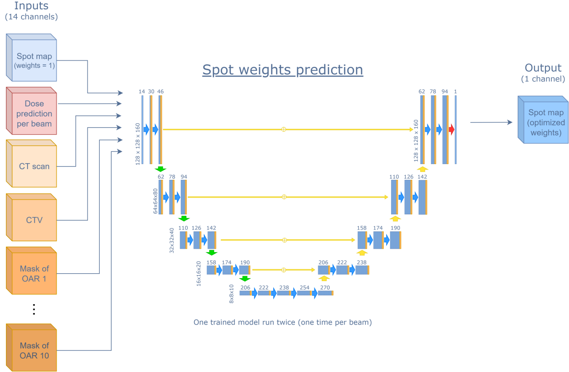
Figure 4.2: The architecture of the HD U-Net network predicting the weights of the spots. The legend for the different operations employed in the network is the same as above (Figure 4.1).
