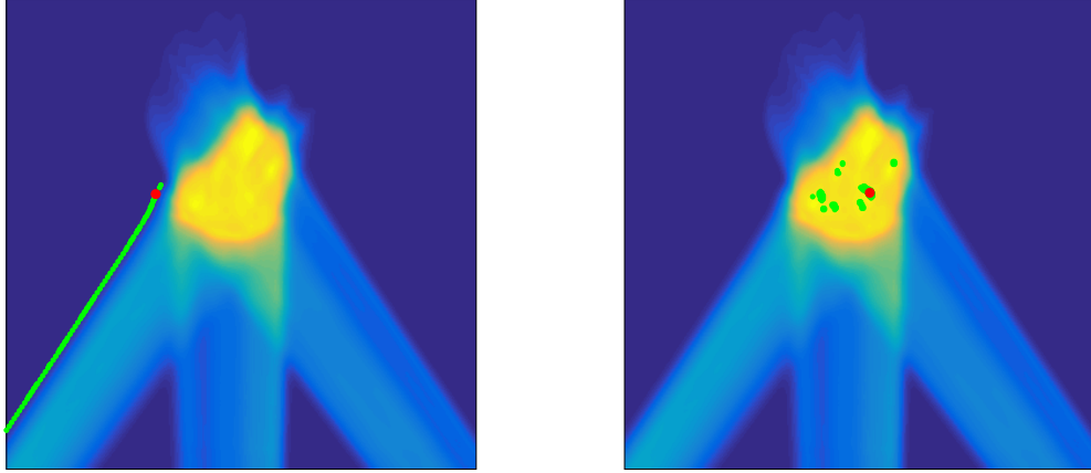
Figure 4.6: Example of similar pixels selected using the vp-tree. The green dots are the 100 closest neighbors of the red dot.
