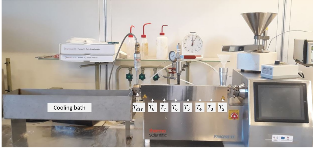
Figure 3.3: Picture of the Thermo Scientific Process 11 Twin-screw Extruder used.
