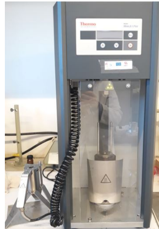
Figure 3.5: Picture of the Thermo Scientific™ HAAKE™ MiniJet Pro used.
