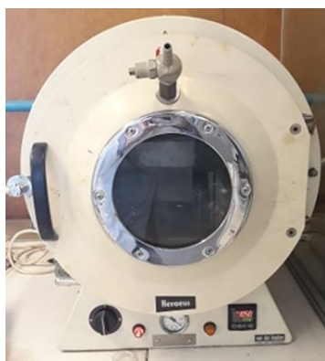
Figure 3.1: Vacuum pump chamber used for drying.
