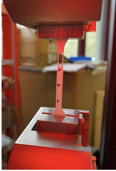
Figure 5.20: Fracture of the PLA/PEO1M blend during the tensile test
