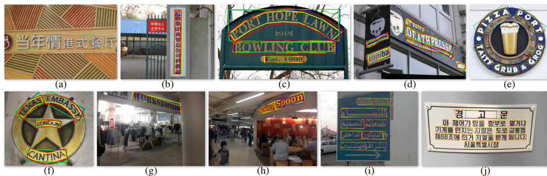
Figure 2.1: Visualization of LOMO’s detection results on challenging images. The yellow polygons are ground truth annotations. The localization quadrangles in blue and in green represent intermediate detection results. The contours in red are the final detection results of LOMO
