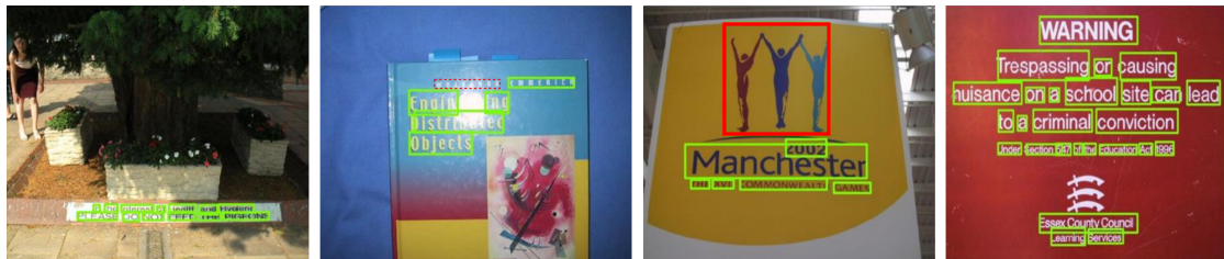
Figure 3.7: Examples of text localization results. The green bounding boxes are correct detections; Red boxes are false positives; Red dashed boxes are false negatives.
