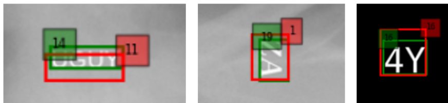
Figure 5.1: Visualization of predicted text boxes (red) with an IoU around 0.5 compared to ground truth (green) during evaluation using COCOEval
