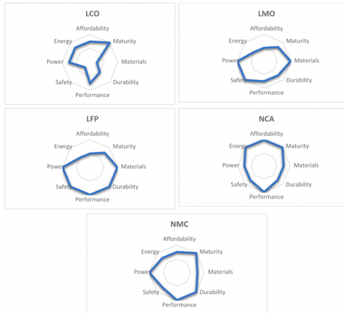
Figure 1-6 Cathode materials for commercial Li-ion batteries [1].
