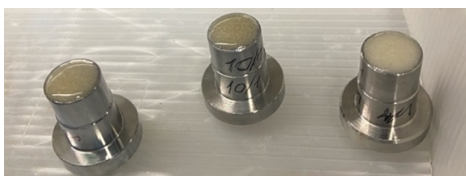
Figure 3-1 Different ratios of G44 / LiTFSI based non-cross-linked electrolytes.
