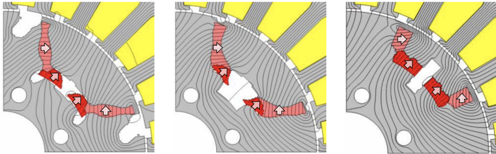
Figure 3.10: Different resultant rotor shapes: the light red and darker red regions represent magnets with different remanent flux orientation. [13]
