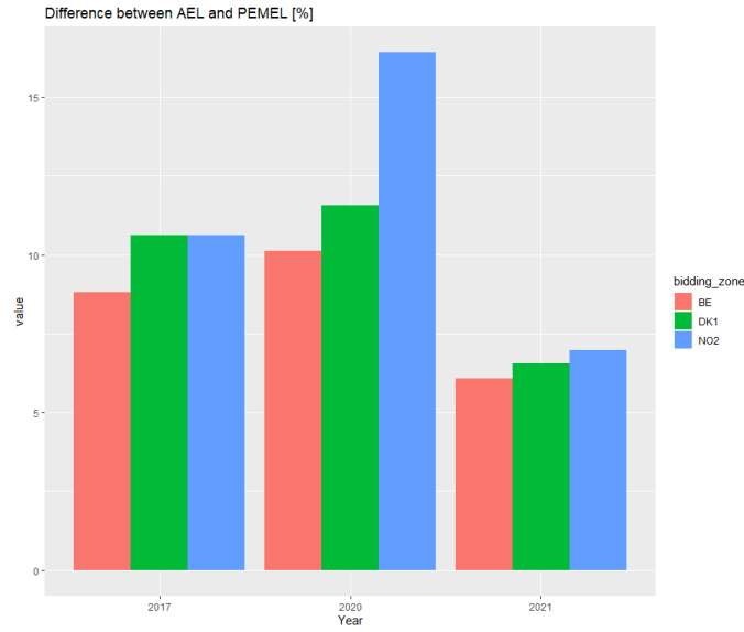
Figure 20: Difference [%] in the Levelized Cost of Hydrogen between AEL and PEMEL
